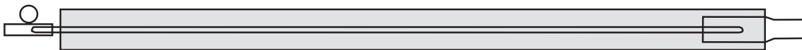
Part# C-1 (Quantity 4) - 44" Long - End Pole Assembly Metal Fitting/Ring & Fiberglass Rod with Foam Pad & Swaged Tubular End
