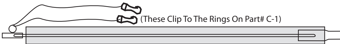
Part# C-2 (Quantity 2) - 44" Long - Middle Pole Assembly Metal Fitting/Ring & Fiberglass Rod with Foam Pad & Swaged Tubular End & Rope Hook Tie (These Clip To The Rings On Part# C-1)
