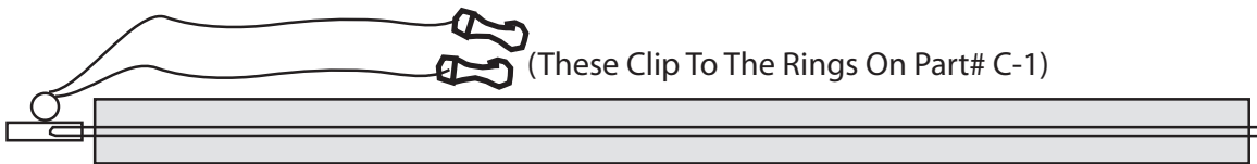
Part# B-2 (Quantity 2) - 44" Long - Middle Pole Assembly Metal Fitting/Ring & Fiberglass Rod with Foam Pad & Rope Hook Tie (These Clip To The Rings On Part# C-1)
