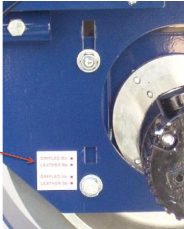
Three of the four slots for the Motor Mount Bolts are elongated completely. The bolt (near the STICKER) is used to set the location of the Motor Mount. As indicated, the upper of the two short slots is for Baseball. The lower of the two slots is for Softball.
